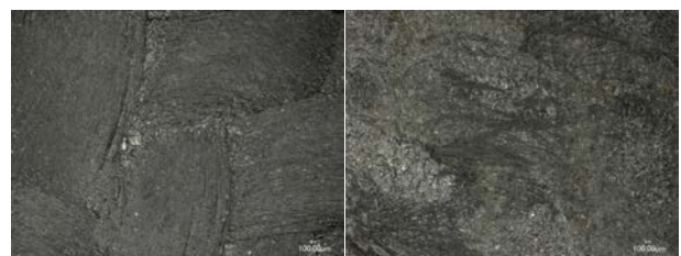
(a) CF/PA6 破断面、×50 (b) A5052(BT)破断面、×50
