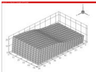
図8 全体構造の変位 (×50、以下同様) Fig.8 Deformation of global structure (×50, the following figures are same magnification)
